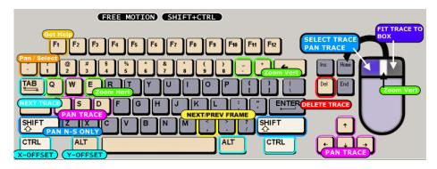
Figure 7.1 Pressing the spacebar brings up keyboard and mouse shortcuts.
