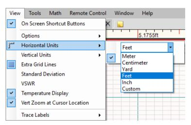
Figure 5.19 The Horizontal Units option is found under the View menu.
