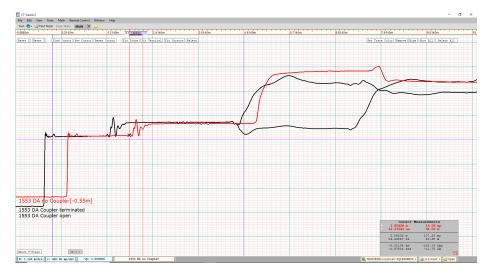
**Figure 4.5** The selected cable has been moved 0.55 meters right from its original position.
