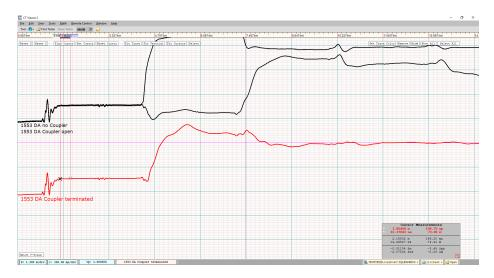
Figure 5.4 Use Shift-S to move only the selected trace down relative to the other traces.
