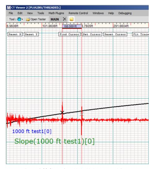
Figure 5.39 Slope of a cable highlighting some defects.
