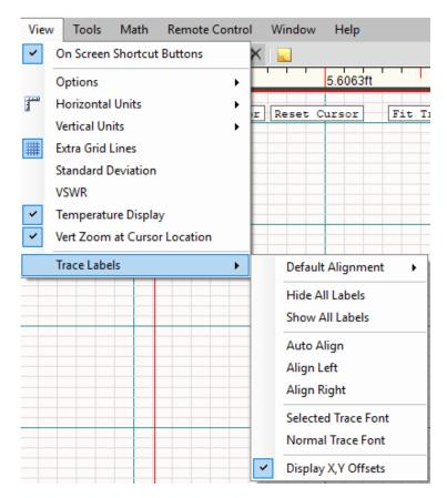
Figure 5.27 The Trace Labels options can be found under the View menu.
