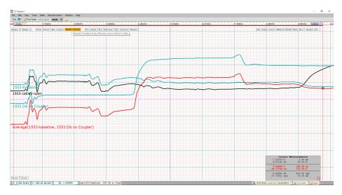
**Figure 5.33** Taking the average of the two teal traces. The new average trace is shown in red.
